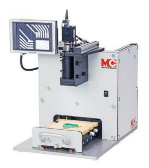
The microtester **MCit** is a manual test system for one-sided - optionally also double-sided - testing of assembled and bare substrates. The substrates are fed manually. The position can be precisely adjusted in the X and Y axis as well as in the rotation with the help of the camera system and the adjustment screws. The contact is made automatically by means of a pneumatic lifting axis.
